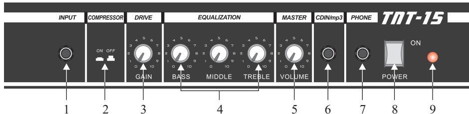
1、**Input** : Socket provided for connecting electric bass guitar..
